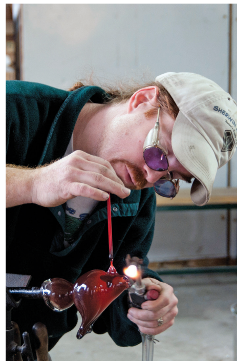
Chris Sherwin creates a glass cardinal using a lampworking technique.
